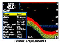
**Scroll**—adjusts the rate that the sonar screen scrolls from right to left. If you are sitting still or the sonar screen is moving too fast, slow the scroll rate or pause the scrolling.
