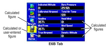
**Indicated Altitude**—required entry for density altitude/true airspeed calculation. Enter the aircraft's altimeter reading.
