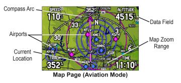
A navigation arc (Horizontal Situation Indicator, or HSI) appears by default on the Map Page. The arc works like the compass on the Panel Page, indicating the course and your deviation left/right of this course. If the route line and magenta arrow are heading straight up, you are heading directly to your destination.
