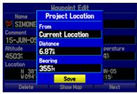
Project Location Menu Enter the distance, bearing, and location to project from. 6. To change the location from which you are projecting the new waypoint, highlight the **From** field, and press **ENTER**. The Find Menu opens.
