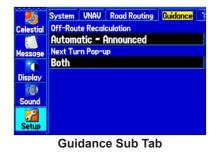
**Off-Route Recalculation**—allows you to set whether the unit prompts you when it is recalculating your route (**Prompted**), or whether the unit recalculates automatically. You can also set whether the unit announces the recalculation (**Automatic - Announced**) or recalculates silently (**Automatic - Silent**). You can also turn route recalculation **Off**.
