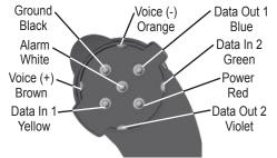
Power/Data Connector on the GPSMAP 296 Unit
