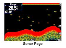
Generally speaking, if the only thing between the transducer and the bottom is water, the first strong return comes from the bottom directly below the transducer and sets the bottom level. Weaker secondary returns provide the detailed data. Stronger returns screen in darker colors, with red being the strongest return.
