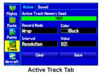
**Record Mode—Wrap** records over the oldest tracks when the track log reaches 100%. **Fill** records a track log until the track log is full (100%). When **Off** is selected, the unit does not record tracks.
