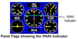
VNAV indicators also appear on the Map Page when the page layout is set to **Map With Overlay**. You are at the proper altitude for the VNAV profile when the blue bars are centered within the VNAV indicators.
