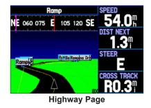
When you are navigating, the Highway Page provides digital and graphic steering guidance to the destination. The right side of the Highway Page features user-selectable data fields showing useful navigation information. A compass ribbon appears at the top of the page to show your current heading as the violet bar and a red vertical bar indicates the bearing to your course.
