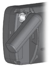
Removing the GPS Antenna
