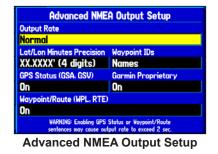
The Advanced NMEA Output Setup Page allows you to set the output rate, change the precision of the Lat/Lon minutes, set Waypoint IDs to names or numbers, as well as turn on and off the GPS status, the GARMIN Proprietary sentences, and Waypoint/Route (WPL, RTE).
